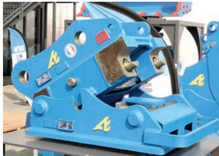
French manufacturer Arden says its new 'all in one' quick hitch – the AIO 50 – will operate with an array of attachments
